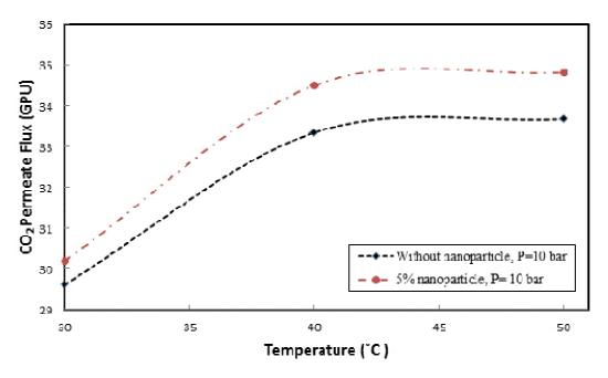
Figure 3. Effect of silica nanoparticle on the CO<sub>2</sub> permeation of the integrally skinned polyethersulfone membrane.
