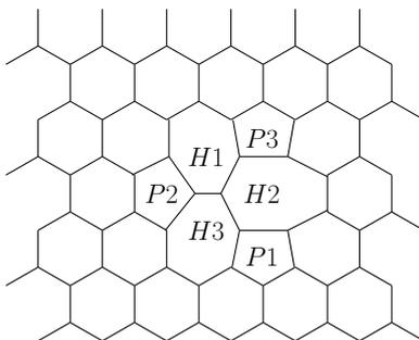
Figure 1: Hexagonal grid with a  $V_2(555 - 777)$  defect
