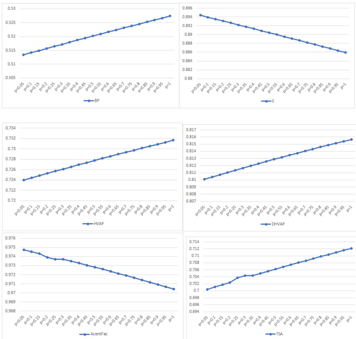
**Figure 3:** Regression line between BP, S, HVAP, DHVAP, AcentFac, TSA of octane isomers and  $SOS_p$  index;  $0 < p \leq 1$ .
