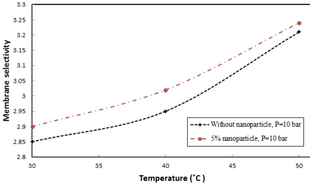
**Figure 4.** Effect of silica nanoparticle on membrane selectivity of the integrally skinned polyethersulfone membrane.
